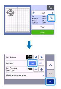
**6** Touch the "Test" key, and cut a trial cutting pattern with the Auto Blade (Black Holder).
