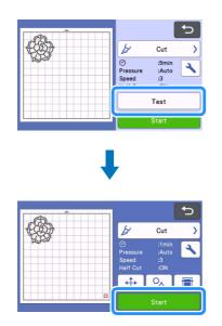
7 If the backing of the template sheet is cut, adjust the Cut Pressure(Half Cut) to lower it.
