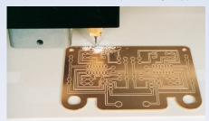
simple 555 based circuit should take no more than a couple of minutes to complete on a RotoCAMM). Virtually any circuit design can be manufactured with this process. It is even possible to put tracks between DIL pads!
