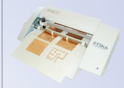
This process, developed by TechSoft, uses a self-adhesive copper foil (Cutronics). This fits into any Roland vinyl cutter and cuts just like vinyl. When weeded, the circuit can be applied to any suitable substrate such as plastic sheet, wood or card. (If card is used it is possible to make bendy, even "roll up" circuits).
