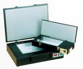
These cost-effective units enable controlled UV exposure of PCB artwork onto pre-sensitised copper-clad board. Both feature a pressure pad in the lid which, when clipped shut, keeps the artwork in close contact with the board for faithful reproduction of intricate designs. Operation could not be simpler. Once the laminate and artwork are in place, exposure time is set on the control panel and exposure is stopped when the time is up.
