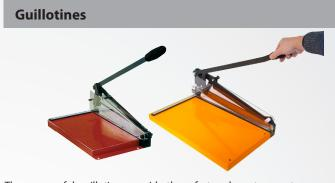
These powerful guillotines provide the safest and most accurate means of trimming PCB laminate to size. Cutting with a guillotine avoids harmful dust, rough edges and blunted blades that result from sawing - especially when working with modern epoxy-glass boards. Safety is ensured by heavy Perspex blade shields and a safety latch to prevent inadvertent operation. Both feature a recessed rule on the bed which aids dimensional accuracy and helps secure the workpiece.
